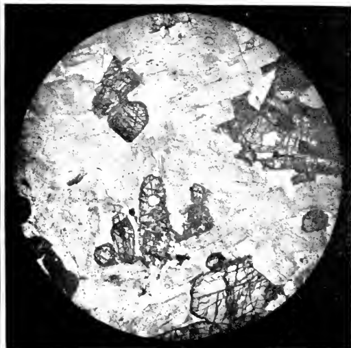
2.—Norite: Creighton mine. Ordinary light X 10. Labradorite pale grey, hypersthene darker grey.
